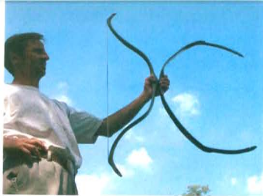
Bowyer Lukas Novotny demonstrates the C-shape of the unstrung recurved bow, which, when strung, takes on its characteristically serpentine, tips-forward shape.
