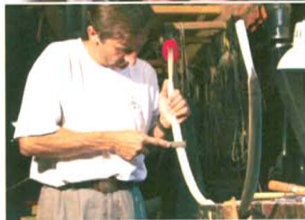
1. Water-buffalo horns await shaving, cutting, steaming and gluing to a wooden core in Novotny's Ohio workshop. 2. Building blocks of a Turkish-style composite bow: two strips of horn, two dustar limbs, two siyahs (attached), a grip and two bundles of sinew; the finished bow at the top shows the final unstrung shape. 3. After gluing horn to the inside of the core, Novotny lays down sinew on the outside of the dustar . 4. He combs the sinew, which will then dry for weeks, pulling the tips of the bow ever closer together. When the bow is curved back, the sinew will be stretched, giving the bow far more power than if it were made only of wood. 5. After a year of seasoning, Novotny uses molded forms called tepeliks to pull the bow into stringing position.
